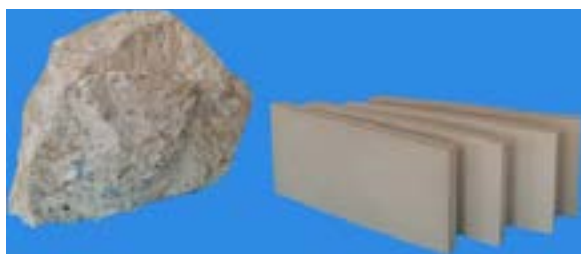
Figure 2 - Albitite of the Aksoran deposit and porcelain tiles based on it
